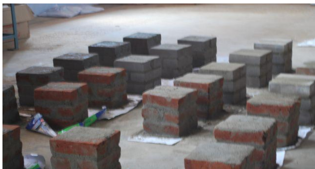
Fig. 1 Casting of Clay brick and Fly Ash Prisms
