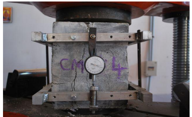
Fig. 8 Modulus of Elasticity Test on Fly Ash Brick
