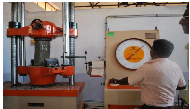
Fig. 3 Test set up for Compressive Strength
