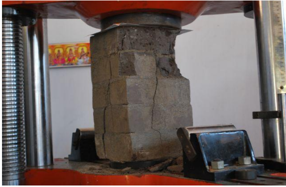
Fig. 5 Compressive Strength Test for Fly Ash Brick
