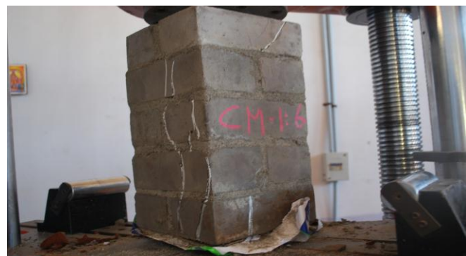
Fig. 4 Compressive Strength Test for Fly Ash Brick
