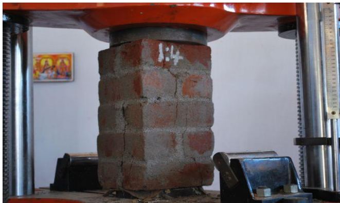
Fig. 6 Compressive Strength Test for Clay Brick
